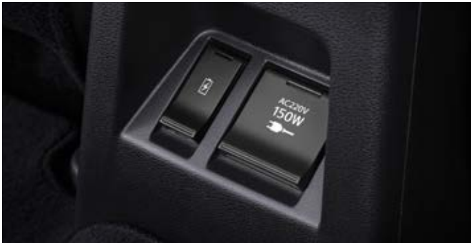
AC POWER OUTLET 220V/150W 1
